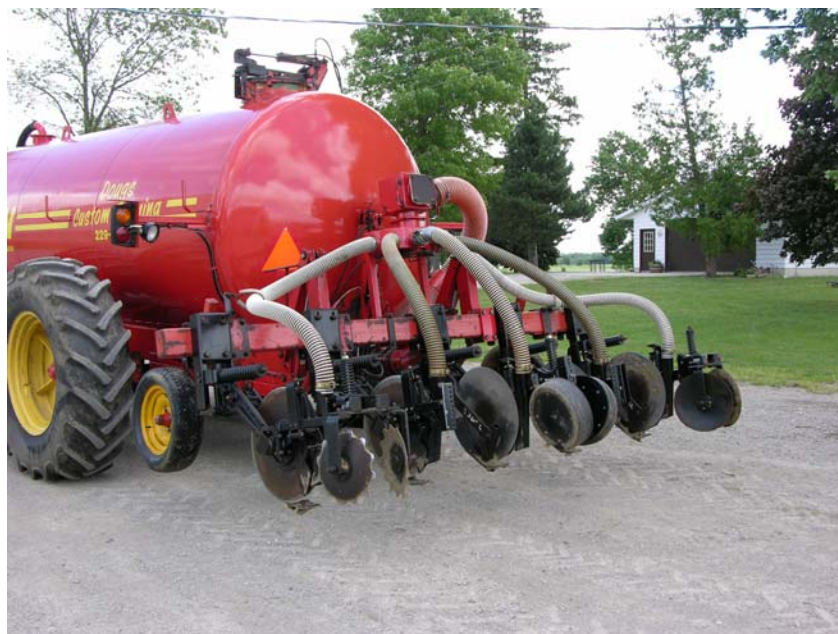
Figure 6. Various Row Closure Attachments on a Yetter Manure Injector
