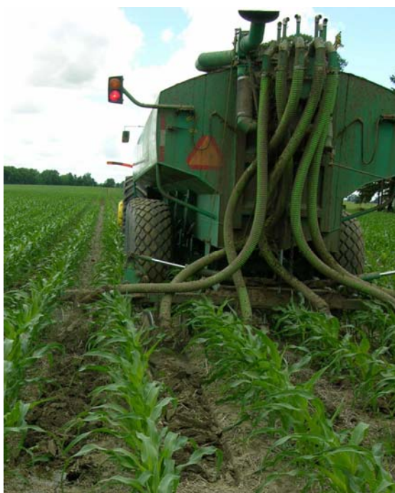
Figure 7. Example of Injector/Row Closure Options Available for Side Dress Manure Application
