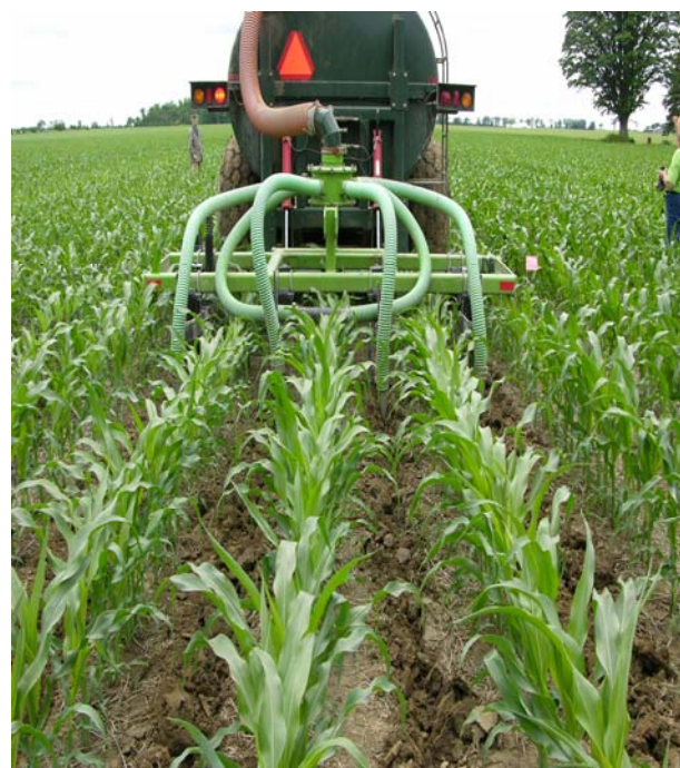
Figure 7. Example of Injector/Row Closure Options Available for Side Dress Manure Application
