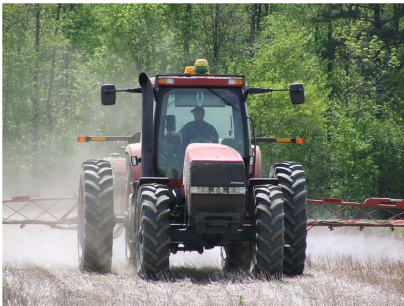
Sprayer Unit and Tractor with Auto Steer
