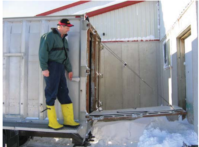
Truck with Catwalk & Adjustable Chute
