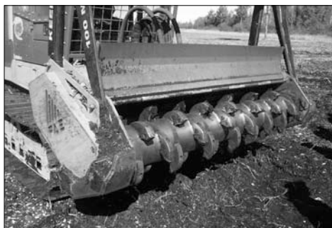
A log and stump mulcher in the forestry exhibit demonstrates new technology that turns a forest into a field in 3 passes.
