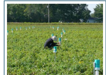
Use rain gauges or catch cans located strategically across the field to measure the actual depth (and volume) of water applied to the crop and the evenness of the application.
