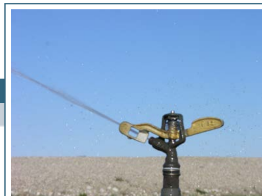
Inspect the sprinkler nozzles yearly. Measure the opening of the nozzle to check if it is worn down. If it is out of tolerance, replace it.
