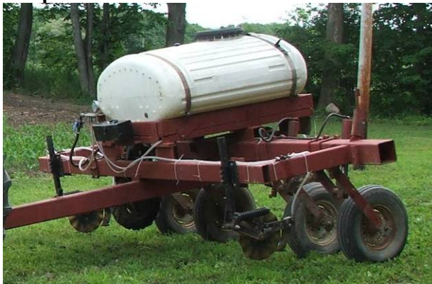
Figure 1. Custom Build Six Row Nitrogen Applicator with Three Fertilizer Coulters Adapted from a Used Corn Planter.
