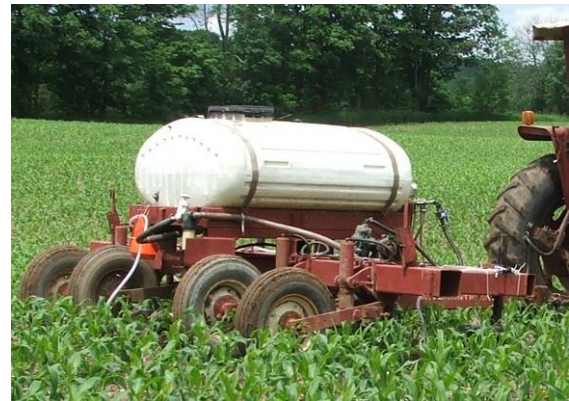
Figure 1. Custom Build Six Row Nitrogen Applicator with Three Fertilizer Coulters Adapted from a Used Corn Planter.
