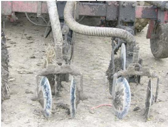
Figure 3. Injector knives (Yetter) with covering discs on manure tanker (Fullarton Site).
