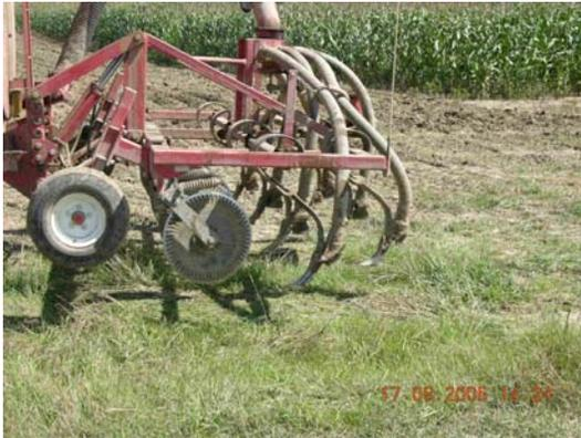
Figure 1. S-Tine injection system on a Nuhn manure tanker (Lucan Site)
