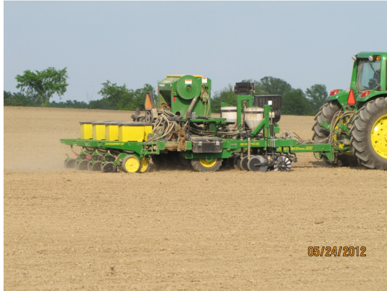
Figure1. 15” row unit planter equipped to apply both liquid and dry fertilizer.
