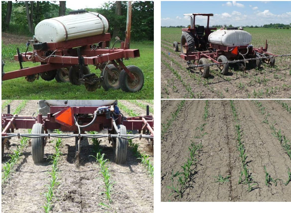
Figure 1. Custom Build Six Row Nitrogen Applicator with Three Fertilizer Coulters Adapted from a Used Corn Planter.
