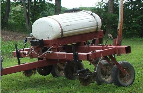
Figure 1. Custom Build Six Row Nitrogen Applicator with Three Fertilizer Coulters Adapted from a Used Corn Planter.
