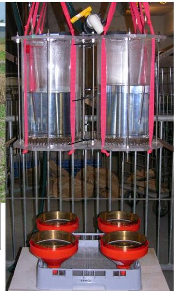
Mega Dripper for aggregate stability testing.
