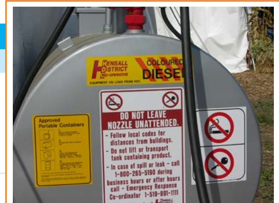
Fuel suppliers can provide proper signage for fuel storage tanks.
