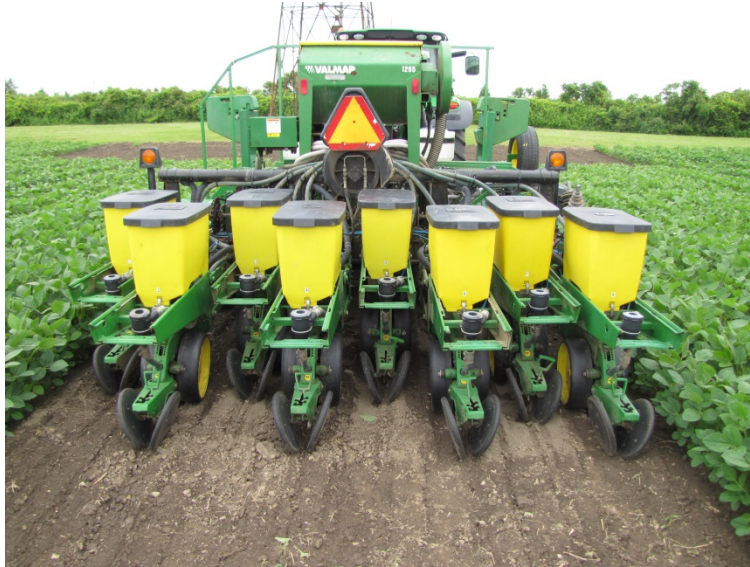
Image1. 15" row unit planter equipped to apply both liquid and dry fertilizer used in 3 of the 4 sites.
