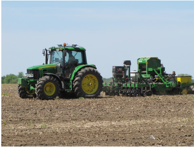
Image 1. 15" row unit planter equipped to apply both liquid and dry fertilizer.
