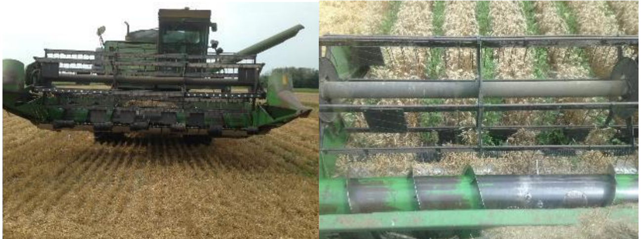
Figure 2: Header with Tile Covers for Wheat Harvest
