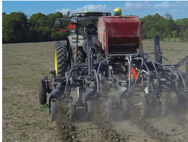
Figure 2. Strip tillage and fertilizer application being conducted in one pass.
