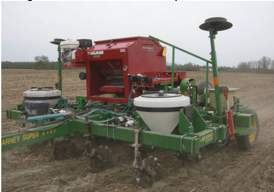
Figure 1: Research planter equipped with liquid and dry starter systems for making accurate treatment and rate comparisons.
