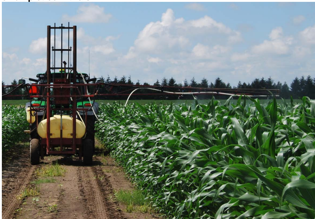
Figure 1. Tow-behind sprayer modified for high clearance applications to small-plot corn trials
