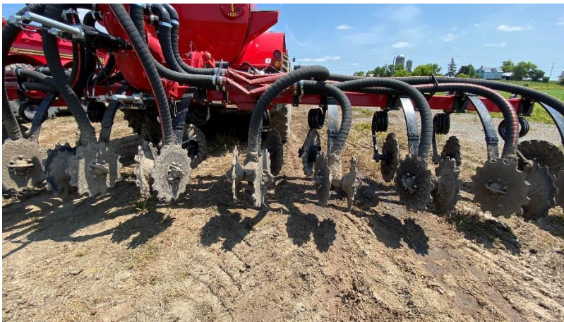
Figure 1: Nuhn Row Crop Manure Applicator used in the project
