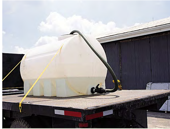
Using a separate tank to supply water to the fertilizer tank will eliminate potential backflow.
