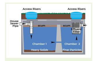
Two compartment tanks retain sludge and scum that otherwise would move into the leaching bed.
