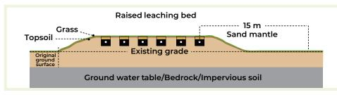
An approved aboveground leaching bed is appropriate where required depth to saturated soil or bedrock is insufficient.
