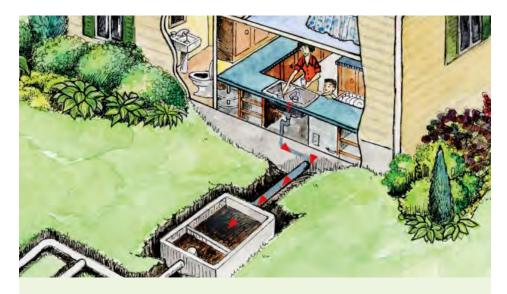
Using a pressure or gravity-fed delivery system, ensure all wastewater, including grey water, goes to a leaching bed.
