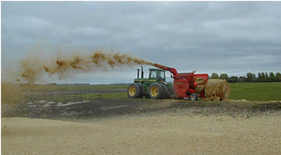
Straw chopper installing a permeable straw cover on a liquid manure storage.
