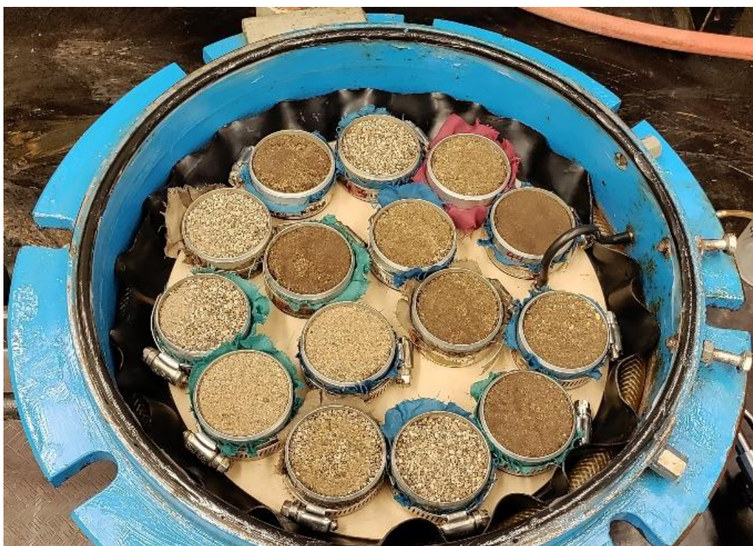
Figure 2. Photograph of soil cores prepared for analysis in the low pressure system.
