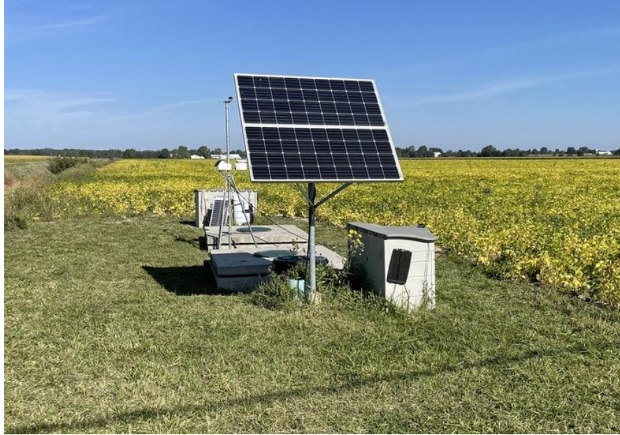
Figure 6. Fairview site containing an inflow and outflow permanent ISCO enclosures with solar panels and a weather station.
