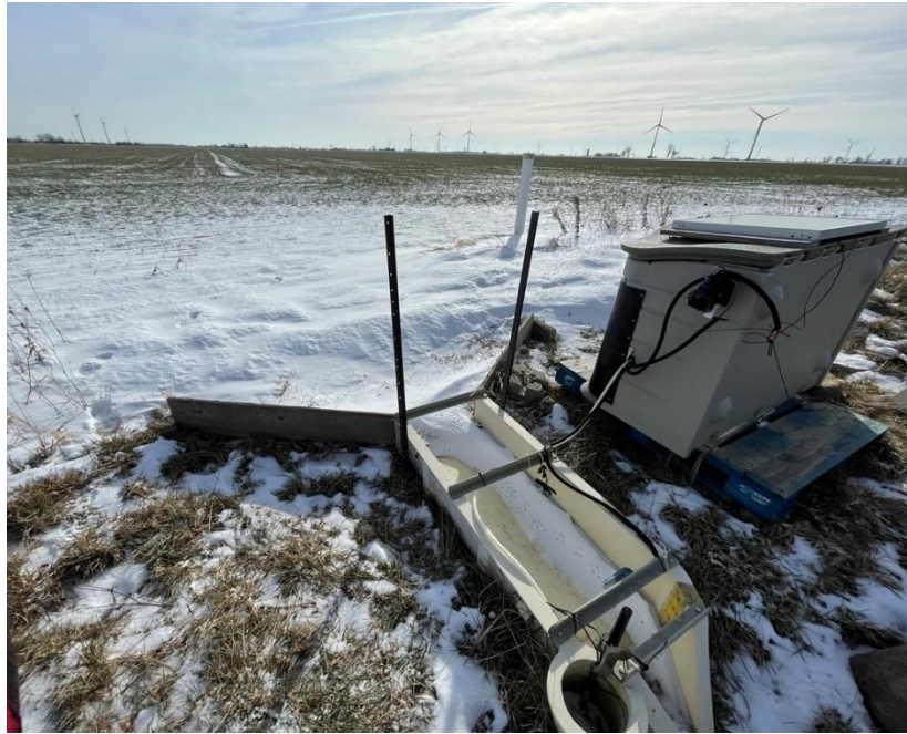
Figure 5. Merlin A site's flume capturing surface flow entering the municipal drain, with the permanent ISCO enclosure.
