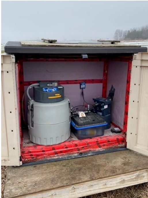
Figure 10. a) Equipment setup at FD: the shed with ISCO autosampler, a Hach water flow meter, and a ZL6 data logger (white box); b) Internal dimensions of the AgriDrain controlled structure at the controlled drainage outlet.
